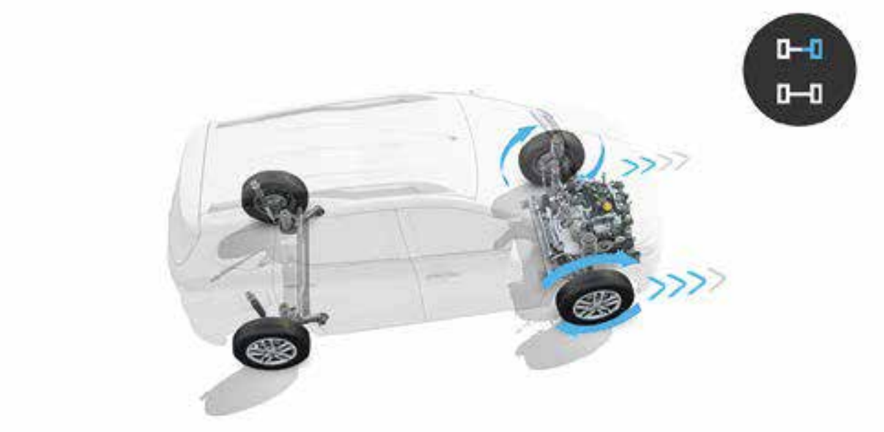
traction control system Limits wheel slip during starting, acceleration and braking.
