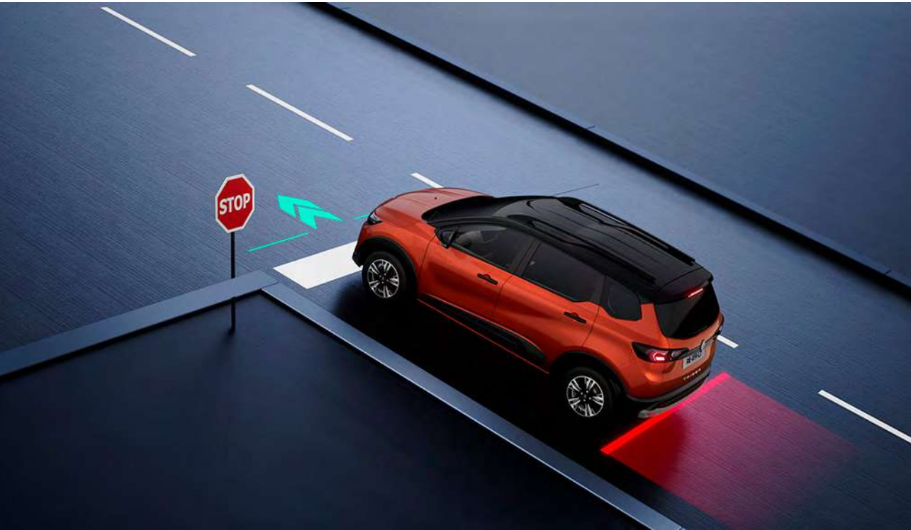
hill start assist Maintains brake pressure for few seconds, preventing rollback when you move away on a steep slope.
