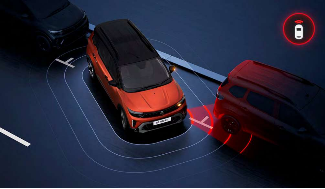
front parking sensors Ultrasonic sensors in the front bumper measure the distance between the vehicle and an obstacle.
