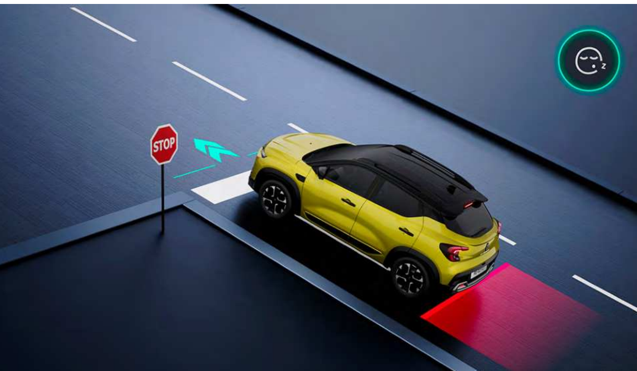
hill start assist Maintains brake pressure for three seconds, preventing rollback when you move away on a steep slope.
