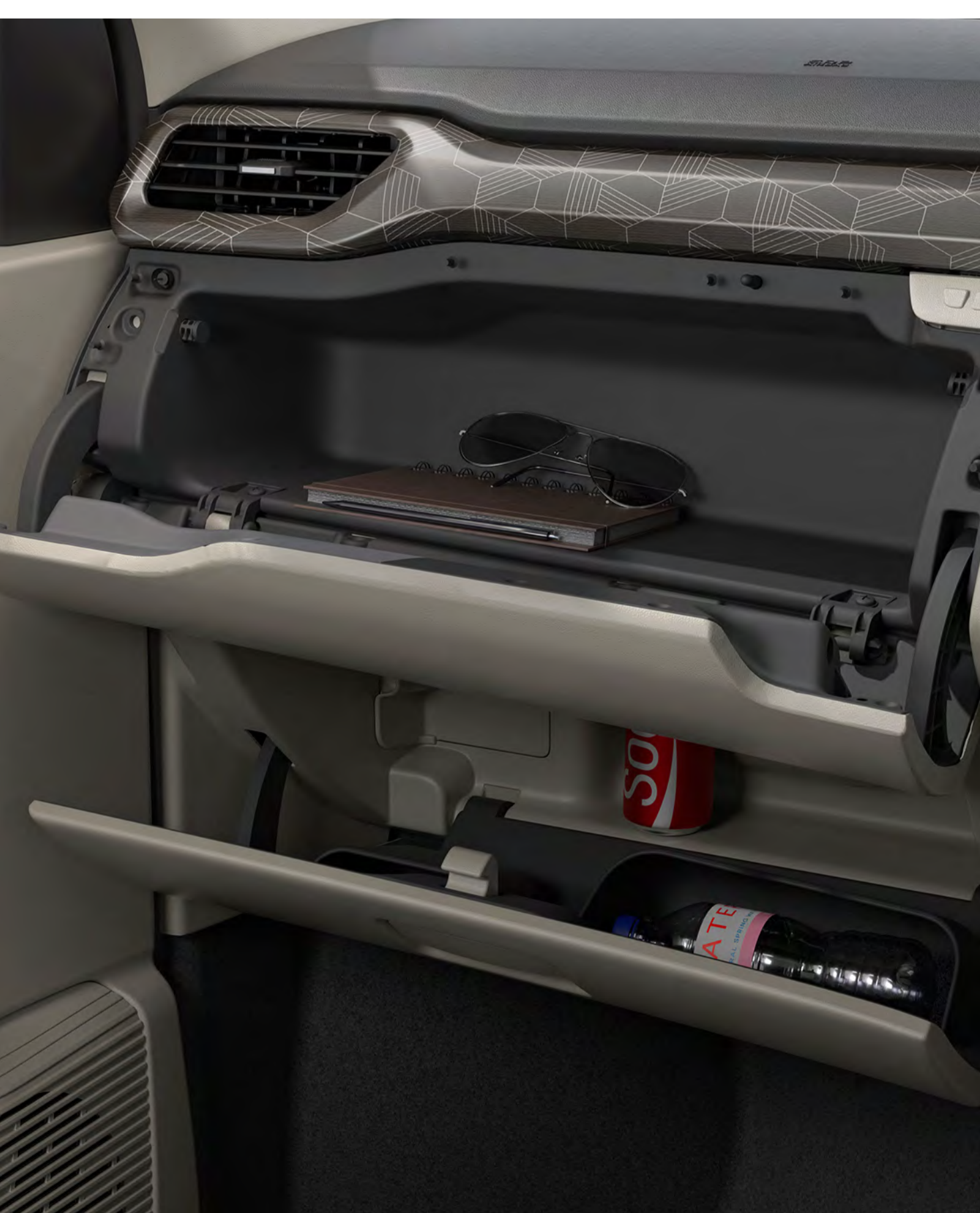
upper glove box & cooled lower glove box
